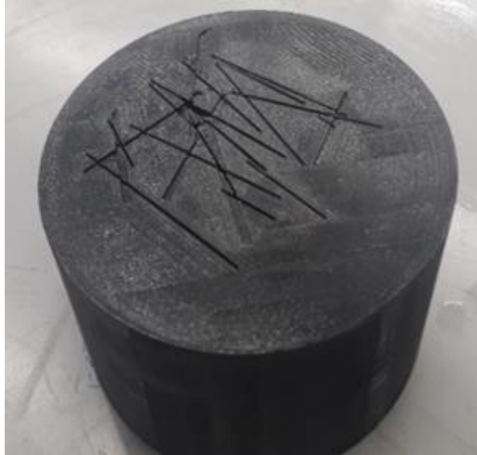
Figure 4.11 3D printed DFN model generated with a Stratasys Dimension SST 1200es 3D printer using ABS material
